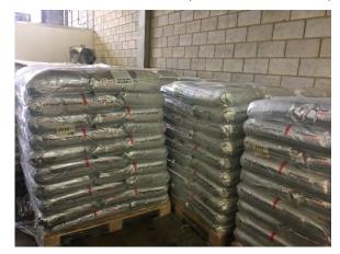
Photo 1. AP-Nylon Caprolactam. Plastic monomer and primary ingredient used in the manufacturing process (McNeall Plastics).
